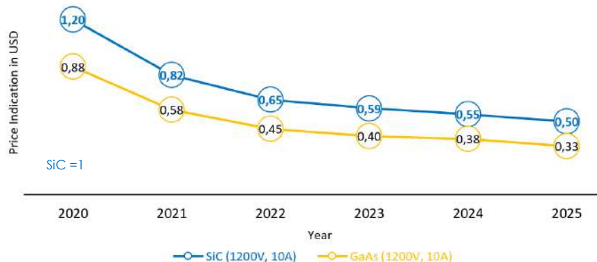
Relative cost of SiC and GaAs 1200V, 10A, Bare die, diced on blue tape at 100Kpcs per Anno
