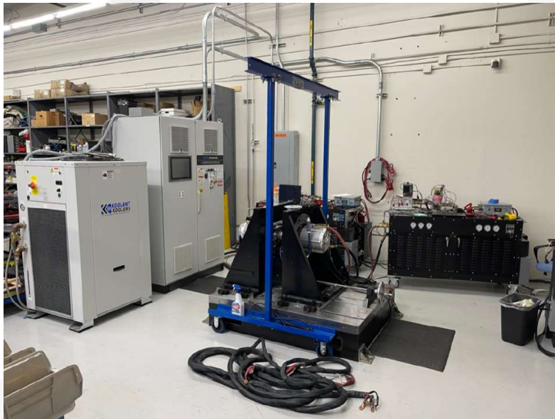
Pre-Switch lab: 250kW 3-Ph AC/DC PSU & Dynamometer
