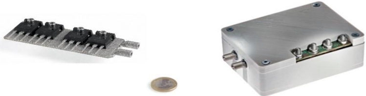
DC/DC converter with 100kW/l:
